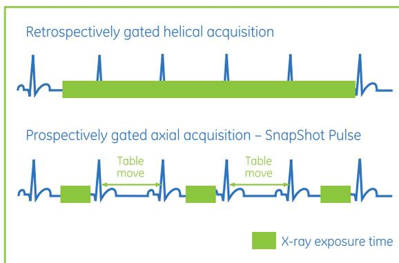
**Figure 18.** Prospectively gated CCTA reduces radiation exposure by >83% with ASiR for heart rates below 65 BPM.
