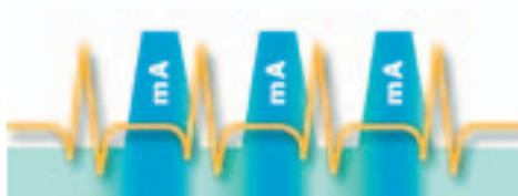
Figure 13. ECG dose modulation achieves up to 50% less dose for most cardiac studies through the use of ECG gating.
