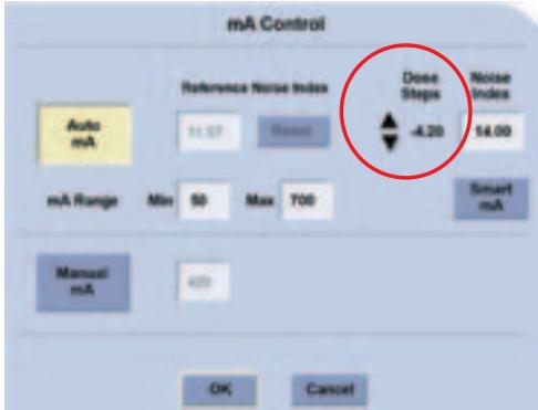
**Figure 9.** Dose Steps – Decreasing dose values increases image noise, thus decreasing the required mA. Each decrease in dose step will increase the NI by 5% and reduce the mA (and patient dose) by about 10%.
